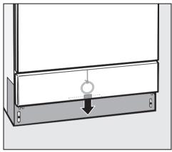
■ Locate the ring for the emergency release cable (at the bottom of the machine, behind the service panel), and pull the ring downward to open the door.
